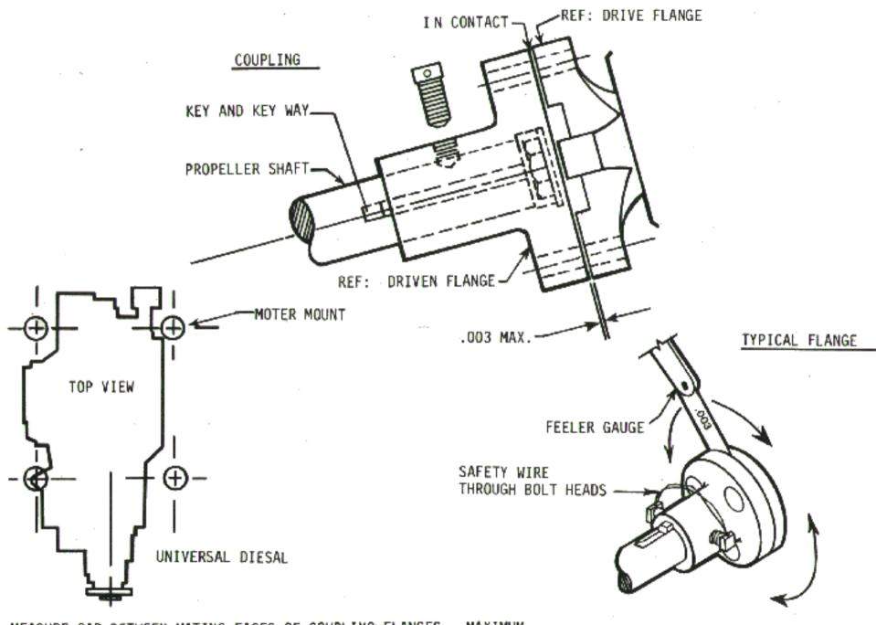
MEASURE GAP BETWEEN MATING FACES OF COUPLING FLANGES. MAXIMUM ALLOWABLE GAP AT ANY POINT IS .003 WHEN ANY POINT OF COUPLING FACES ARE IN CONTACT. TAKE THIS MEASUREMENT SEVERAL TIMES, ROTATING SHAFT TURN EACH TIME. THIS MEASUREMENT MUST BE MADE WITH COUPLING BOLTS REMOVED.
