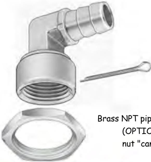
Once tightened up, thru-drill the hose barb and bushing to install small cotter pin. (Belt & Suspenders overkill to prevent the busing from falling into the air intake.)
